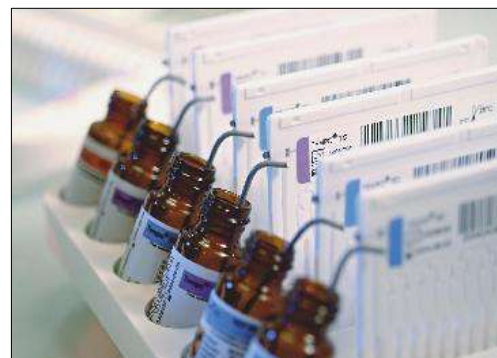
Figure 3. Card with a transfer tube and an ampoule with a specific culture medium.
