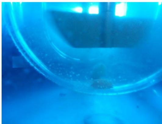
**Figure 1.** Swelling of the tablet by solvent
